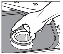
■ To unscrew the micro-fine filter, grasp the two tabs and turn twice counterclockwise.
